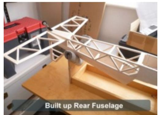
Not knowing how the thing would balance I cut the nose fuselage sides considerably over length, waited until the airframe was complete, taped all the bits & bobs (moving surfaces, esc, etc.) in place and then set about positioning the bulkhead, motor, prop, spinner & battery to get it to balance.
