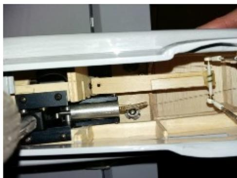
Graham's auto-closing gear door mechanism is little more than a sprung plate connected to the gear doors via short tie-rods, with the gear down the sprung plate holds the doors open and when the gear is retracted the wheel pushes the plate back, overcoming the spring pressure, which closes the doors. Check out the photo, it is a lot easier to comprehend than my explanation! Fine adjustment is made with the tie rods - neat as you like.
