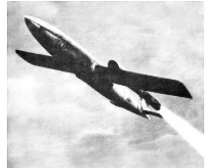
*[These were the Vergeltungswaffe 1 or Vengeance Weapon 1, a small pilotless aircraft powered by a pulse-jet which gave them their characteristic sound. They had a rudimentary distance measuring device that cut the engine and tipped the horizontal stabiliser when over the target so that the bomb came down vertically. Often this did not work and the aircraft flew onward until the fuel ran out and then glided to earth, which is how some managed to reach High Wycombe. (Ed.)]*
