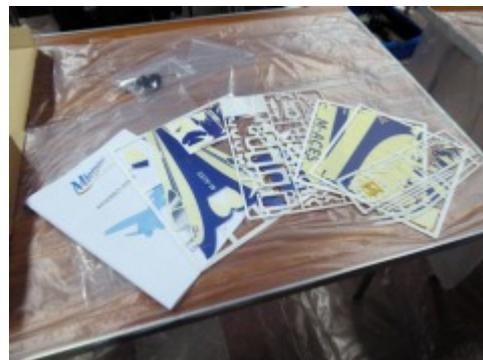
This is because the main structure of the models is made from 2mm Depron foam with a 1mm Depron covering and very thin plastic reinforcement. These are all very cleanly laser cut and look much like a very flat Airfix kit. The printed instructions
