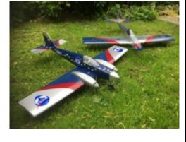
adjustments although the motors may need a bit more down and side thrust as the plane climbs rather too much on power.
